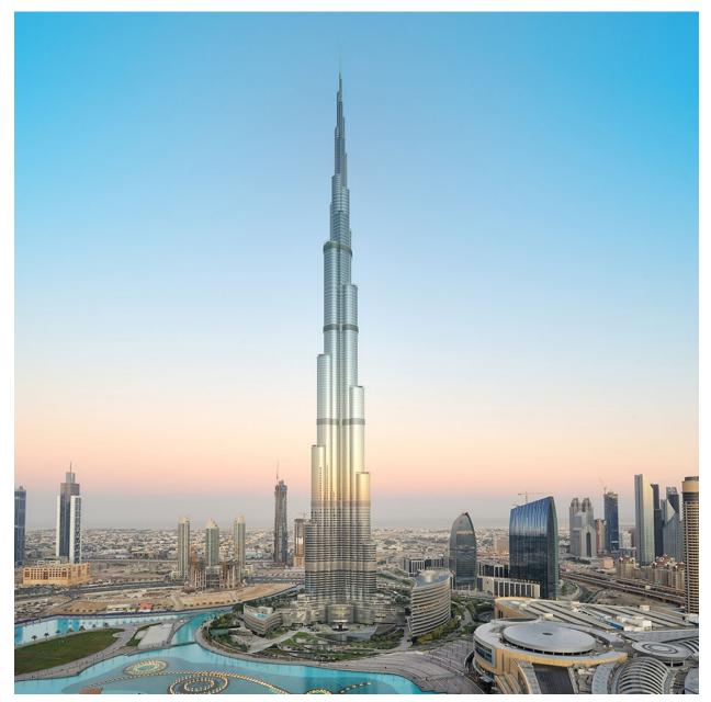
Building a skyscraper in the middle of the desert is no easy challenge. Corrosive salt water running underground between the soil, sand, and rock presented a major challenge for the Burj Khalifa. Engineers had to use special concrete that does not allow salt water to pass through and a process known as cathodic protection in which another metal is added to the concrete base to protect the load-bearing steel beams from corroding if the salt water eats through the concrete.
